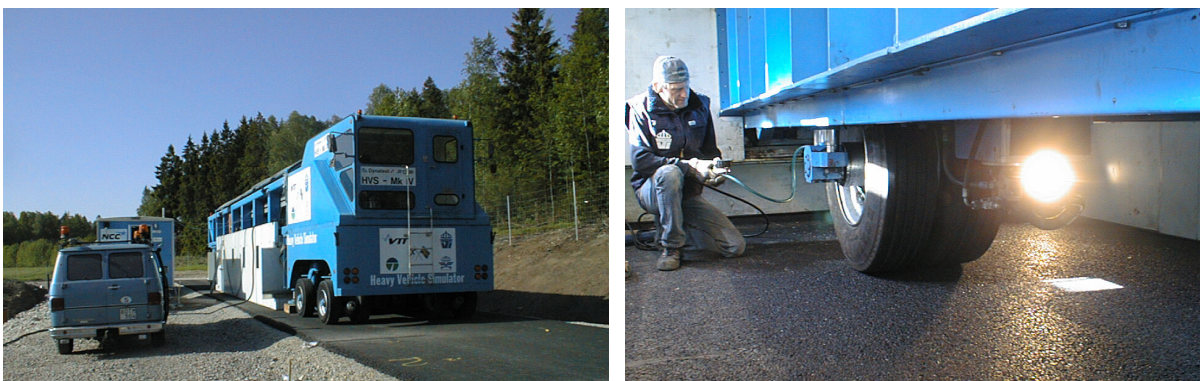
Figure 5.4. The HVS with climate chamber at the test site in Uddevalla. A dual wheel configuration was used during the tests.
