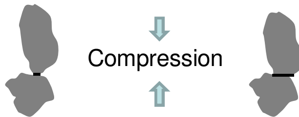
Figure 3.7. Elastic increase in the contact area between the particles due to compression.
